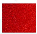
Anti re-entrainment barrier Prevents oil / water carryover and is compatible with a wide range of lubricants.
